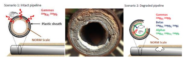
Two scenarios of pipeline assessment (routine operation left and degraded pipeline right) that will be undertaken in the research and an example of the build-up of (predominantly) barium sulphate NORM scale in pipelines
